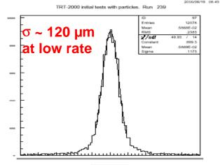
Track-to-measured position residual, mm
