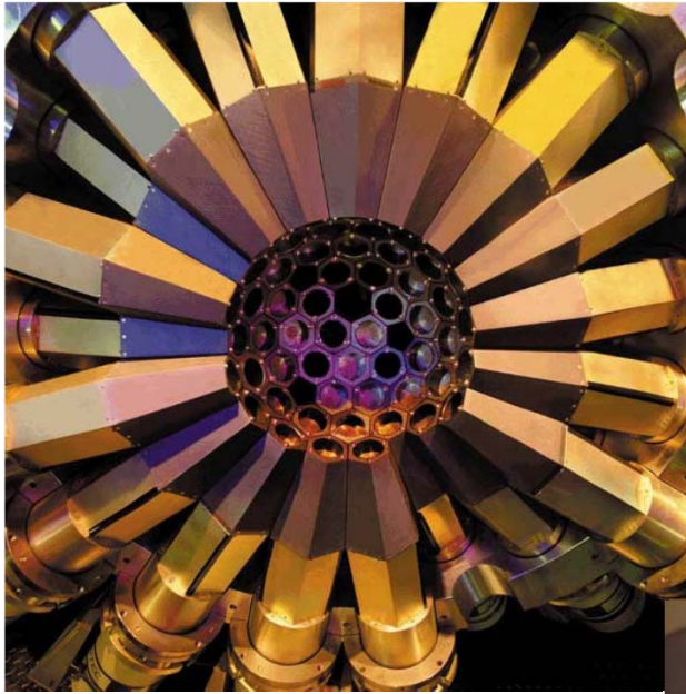
One hemisphere of Gammasphere (51 Ge detectors)
