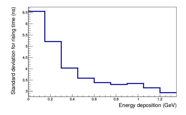
Above 300 MeV energy deposition pulse shape is not sensitive any more to shower profile / preamplifier noise
