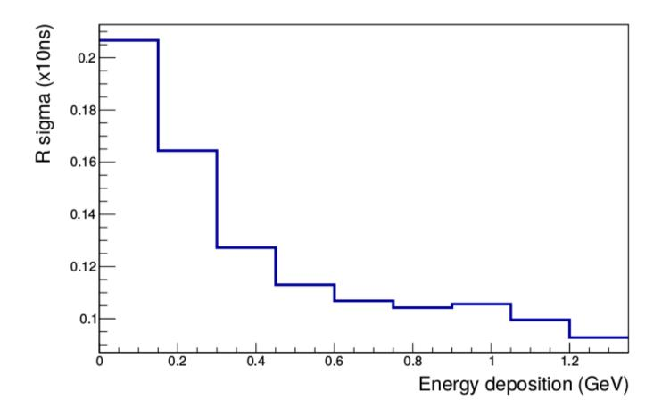
**Definition of rising time:** time within the pulse reaches 90% of its amplitude starting from the 10% level ( = 3.17 \* R)
