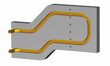
Crates will be mounted between cooling plates, which are simultaneously supporting structures
