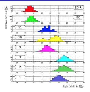
⇒ the larger the level of tapering, the higher the light yield output
