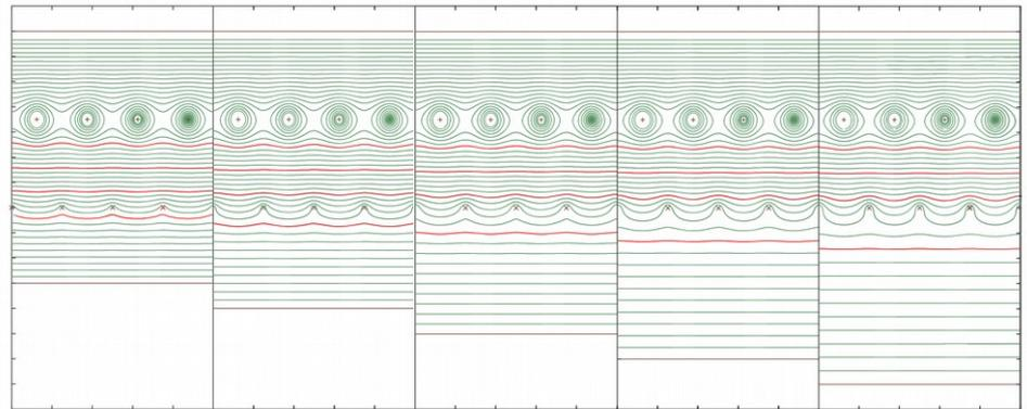
Field distortion by entrance window stretching (Garfield sim.)
