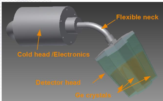
Prototype based on a single-encapsulated-crystal
