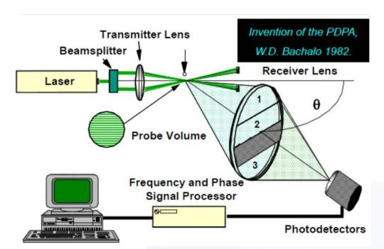
Goals: measurement of size and velocity of droplets/pellets
