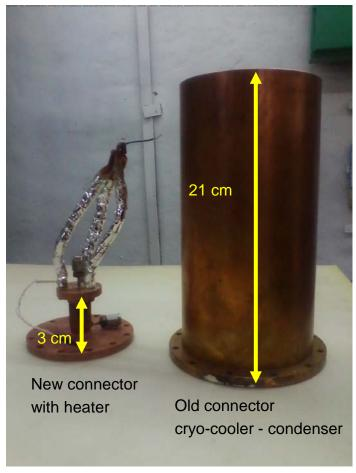
Comparison low temperature tests for two geometries show improvement of the temperature from 20 K to 12.8 K at control point near the condenser
