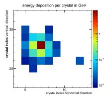
simulation of a 10 GeV photon cluster in the Forward Endcap with split-off
