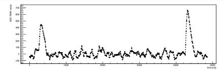
• resulting waveforms  $\longrightarrow$  close to hardware signal
