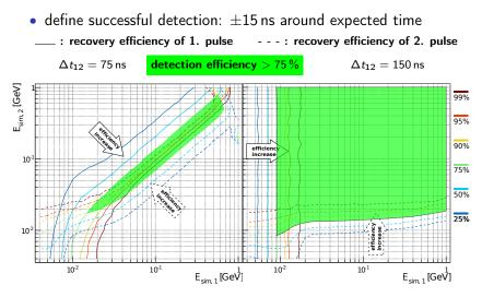
•  $\Delta t_{12} > 100 \text{ ns}$  for almost always successfully detection
