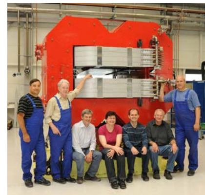
Prototyp of NC-magnet from BINP for testing at GSI
