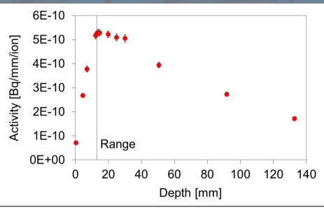
Depth profile of <sup>131</sup>I (T<sub>1/2</sub> = 8 d) primary ion fragment copper irradiated by 950 MeV/u <sup>238</sup>U ions
