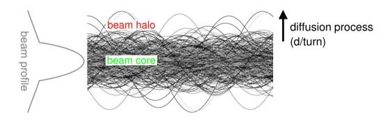
Diffusion speed can be very low: < 1 µm/turn (in synchrotrons)
