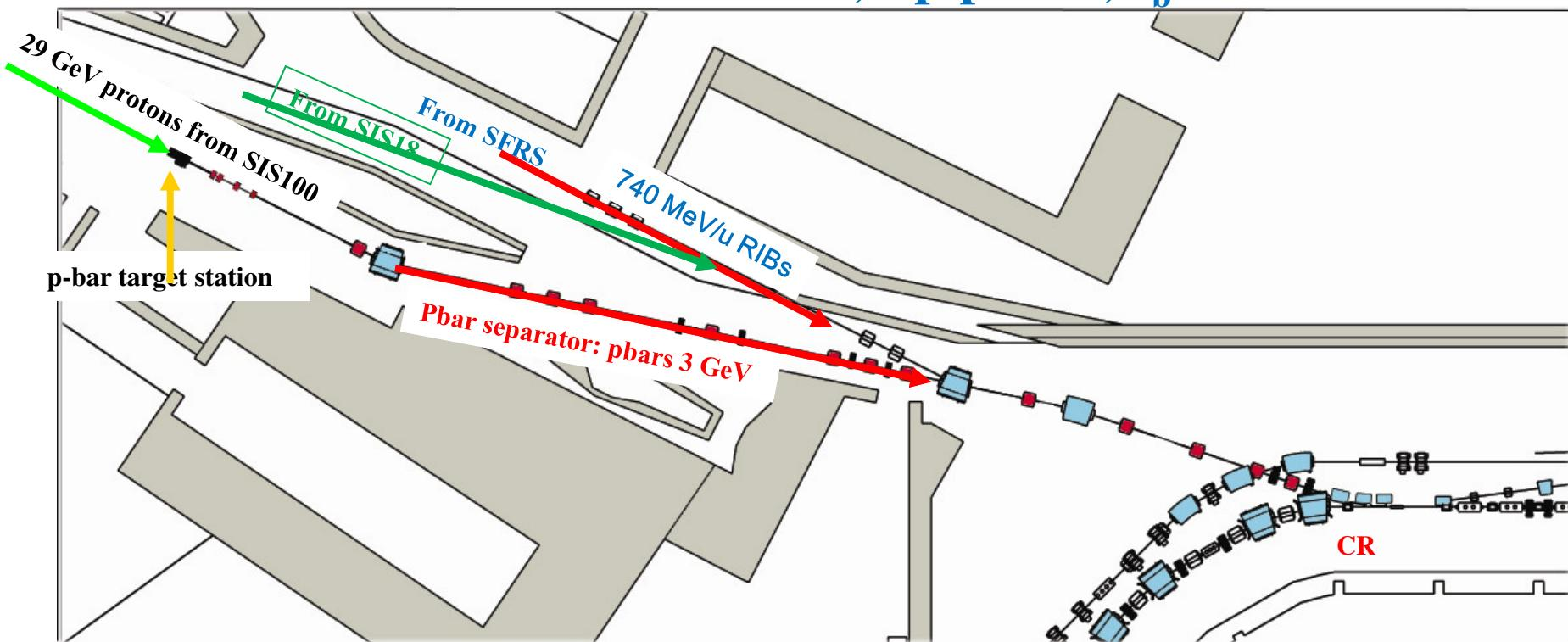
Antiprotons from pbar-sep.: 240 mm\*mrad;  $\Delta p/p=6\%$ ;  $t_b=50$  ns
