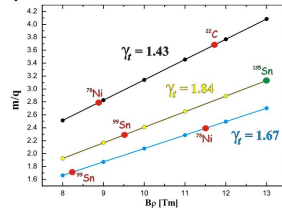
$$\frac{\Delta f}{f} = -\frac{1}{\gamma_{tr}^2} \frac{\Delta(m/q)}{m/q} + \left(1 - \frac{\gamma^2}{\gamma_{tr}^2}\right) \frac{\Delta v}{v} + \left(\frac{\delta f}{f}\right)_{error}$$
