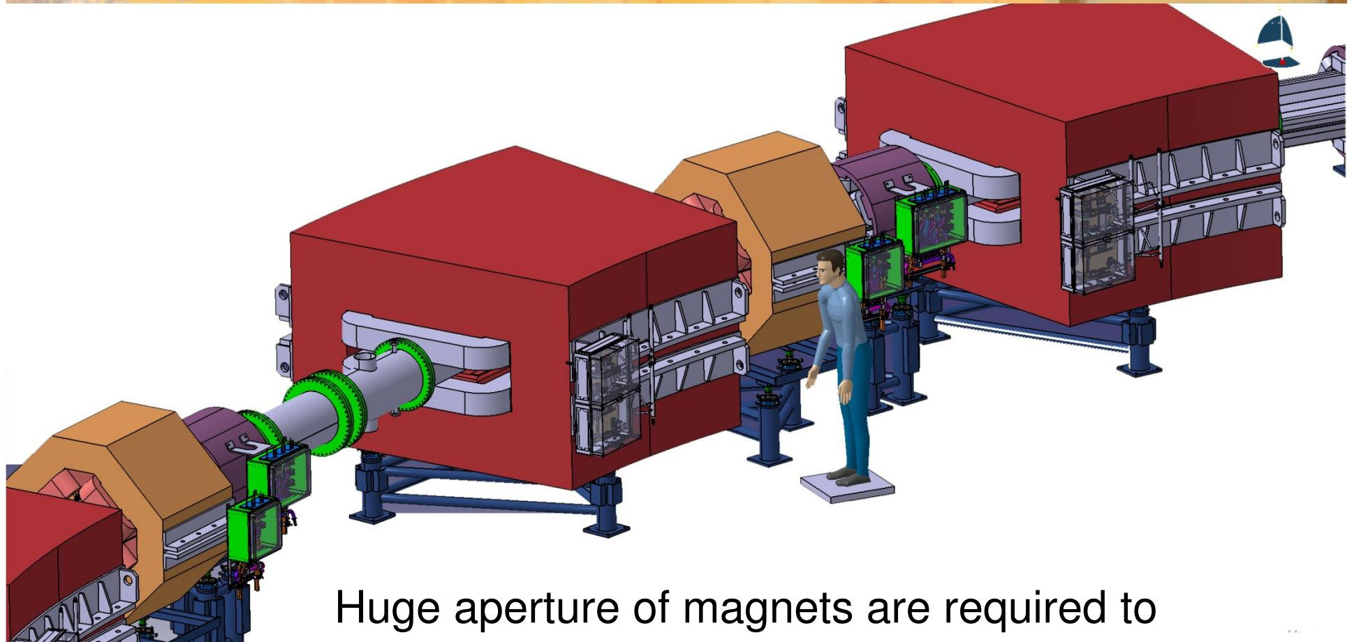
Huge aperture of magnets are required to collect as large as possible the number of antiprotons and RIBs.
