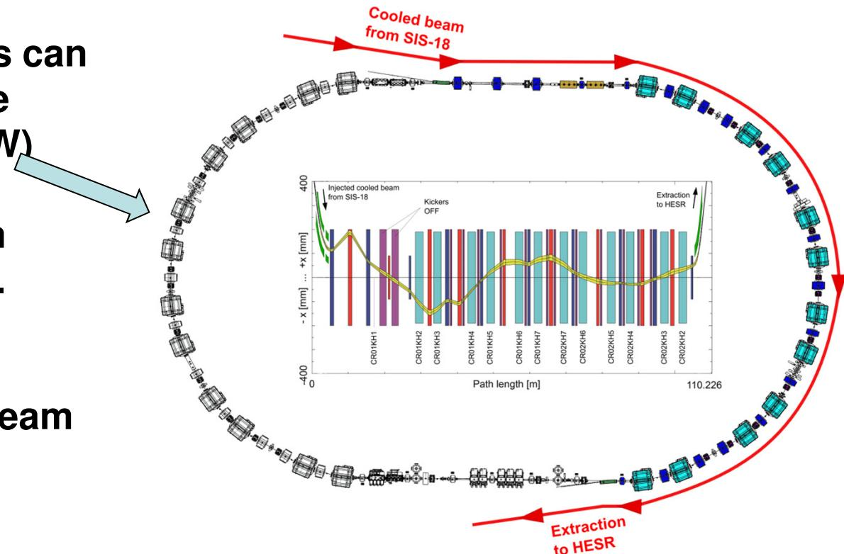
The extraction system of CR is limited by a max. emittance of 20 mm\*mrad
