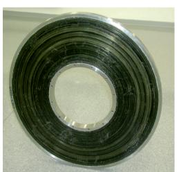
Thin ribbon of cobalt based magnetic alloy (VitroVac6030F) wound to a ring core. Manufactured at VACUUMSCHMELZE Core stabilized by an inner ring of stainless steel.
