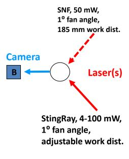
New stronger lasers with variable power allows for measurements of efficiency curves (Nov 14).
