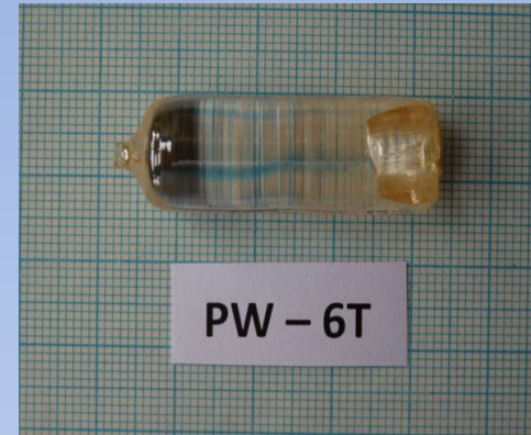
Fig. 1 (a) Photo of \text{PbWO}_4 crystal grown in oxygen-free atmosphere. (b) 50 ppm Y doped grown in air; (c) La+Y doped grown in \text{N}_2+0.1\%\text{O}_2 atmosphere
