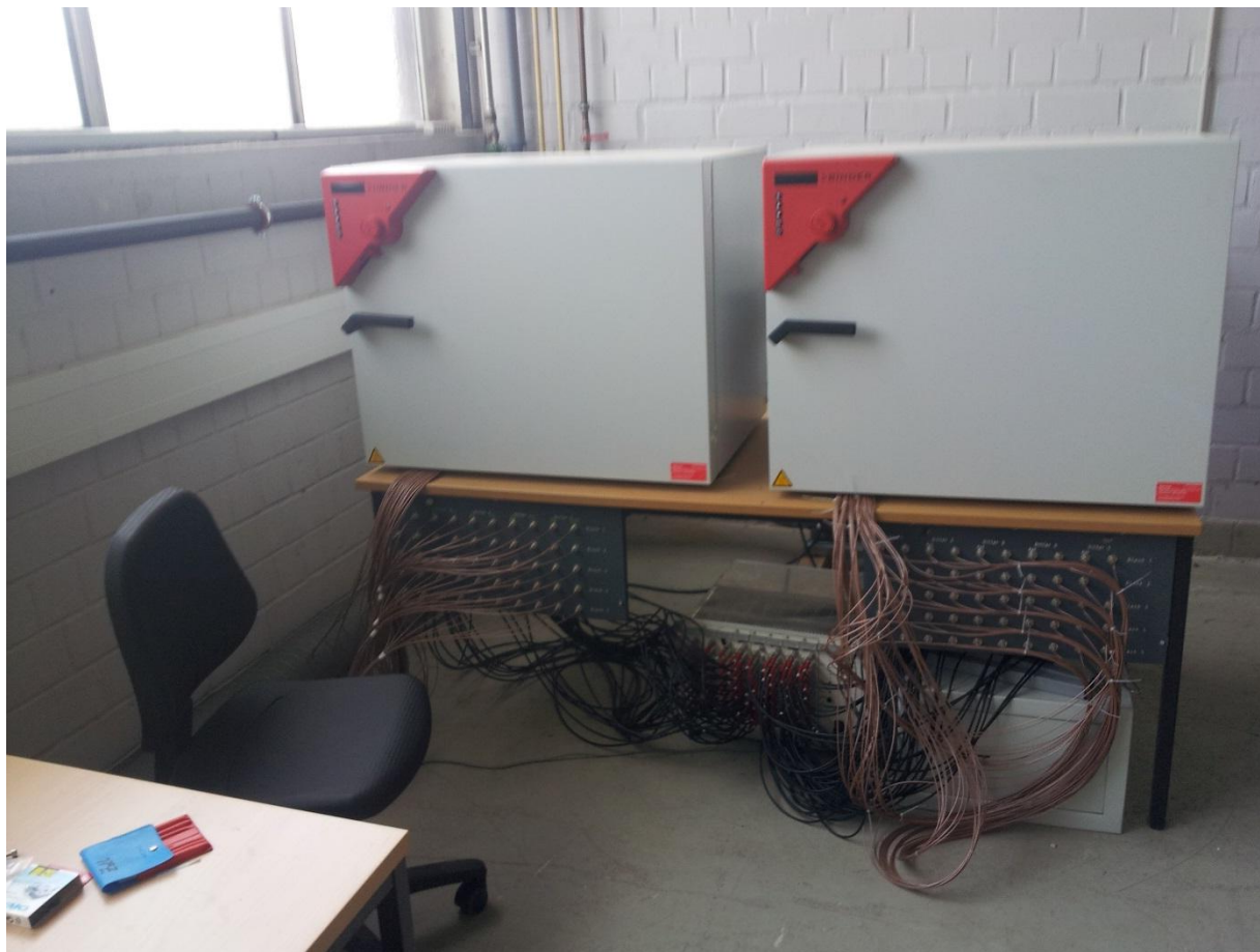
Each Oven: 500 APDs capacity
