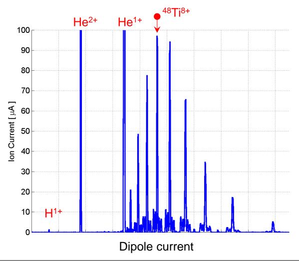
Inj-coil = 1237 A Extr-coil = 1099 A HTO = 10.2 V / 25.6 A f = 14.5438 GHz P<sub>fwd</sub> = 234 W P<sub>refl</sub> = 95 W
