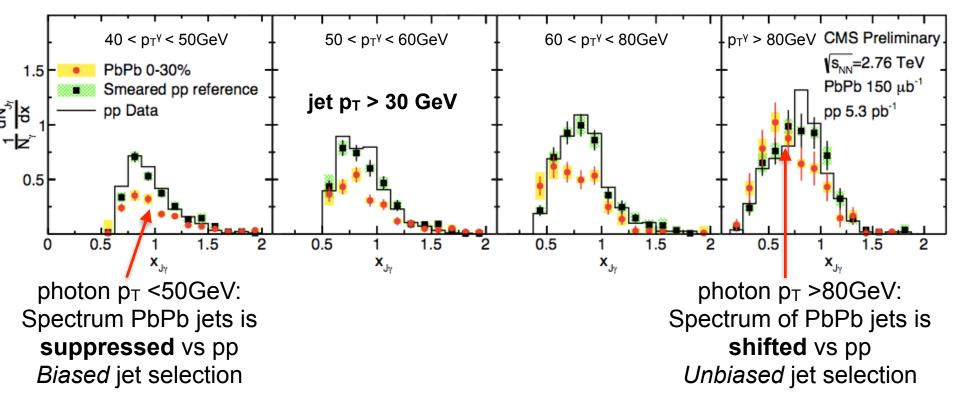
Sufficiently high  $\gamma$   $p_T$  or sufficiently low jet  $p_T$  yield **unbiased** selection of jets
