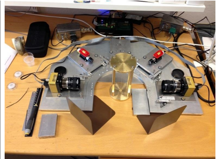
Integrated measurement level with 2 lasers and 2 LS-cameras being aligned in a desktop setup using 5 fishing lines.
