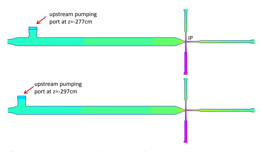
If the upstream pumping port would be placed 20cm further upstream the pressure integral over 16 meters would be 3% higher. In order to compensate this increase the effective pumping speed at the port needs to be 9% higher.
