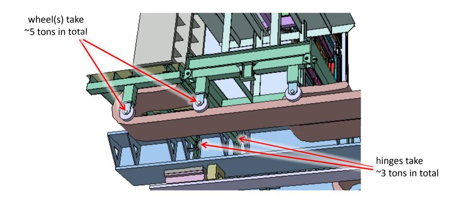
During travelling of the TS between beam area and maintenance area the position of the Bw-EMC has to be monitored and adjusted if the unevenness of the wheel track becomes too big.
