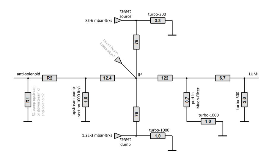
resistor values [in seconds/m³] are reciprocal values of vacuum conductance (resp. pumping speed), hydrogen target with thickness 4.0E15/cm² (outgassing and leaking neglected)
