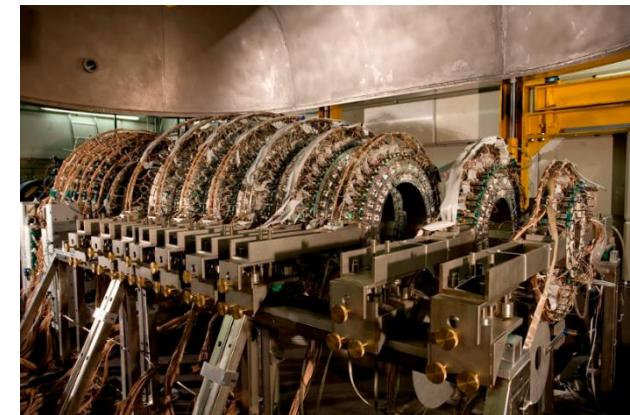
First 3 **forward rings**  $\rightarrow$  144 telescopes ( $1^\circ \leq \theta \leq 7^\circ$ ) complete azimuthal coverage  $\rightarrow$   **$\Delta E$ -E identification** technique.
