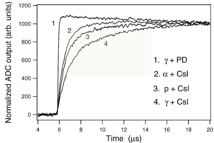
Particle identification in CsI(Tl) using digital pulse shape analysis –
