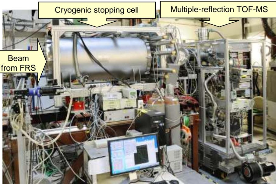
**Successful on-line test** of the **prototype** of the cryogenic stopping cell at the FRS Ion Catcher 2011/2012
