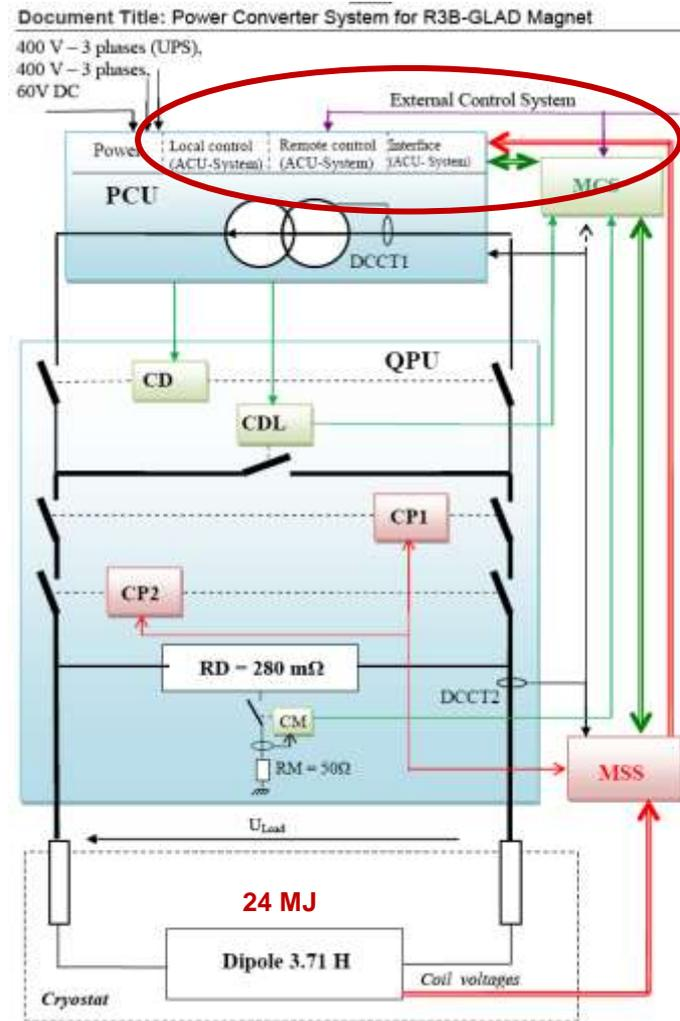
Figure 4 power converter system overview
