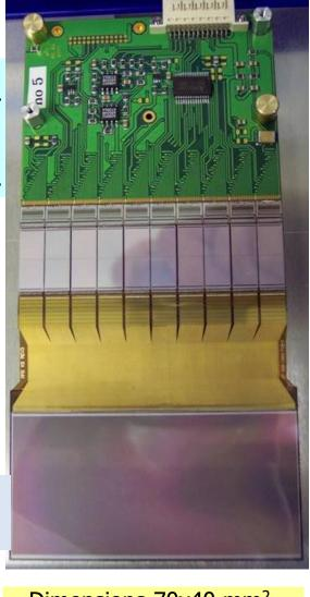
Dimensions 70x40 mm<sup>2</sup>, 0.1 mm strip pitch, in total 1000 channels
