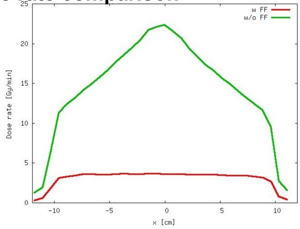
The system (internal ion chambers) measures the dose rate at the edges, only ~3 fold increase
