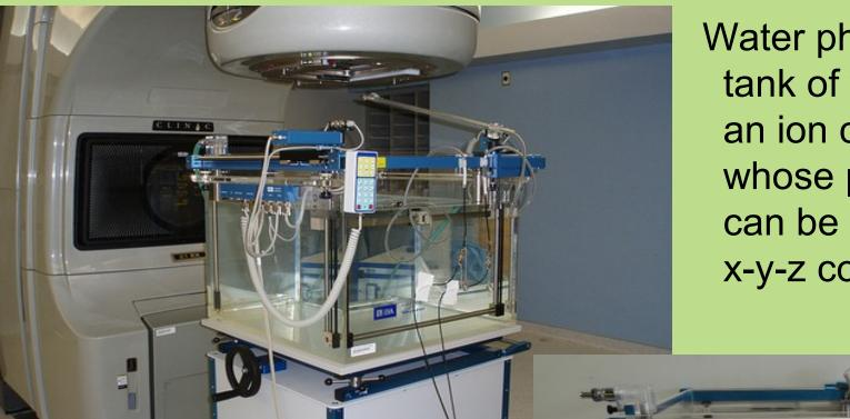
Water phantom is a tank of water with an ion chamber whose position can be changed in x-y-z coordinates
