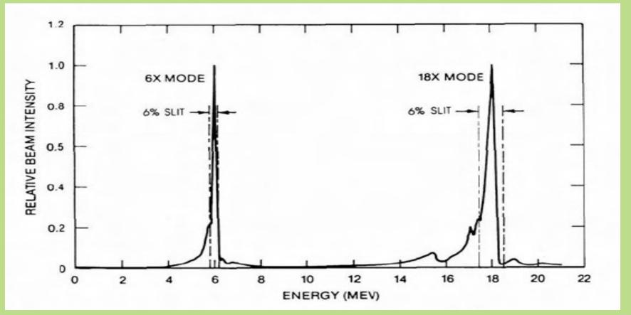
Typical electron energy distribution in an medical linac The allowed deviation of the mean of the energy spectrum transmitted by the energy slit is limited to  $\Delta E/E=1\%$  this is achieved by accelerating with broad electron spectrum ( $\Delta E/E=20$  %) and selecting the narrow energy window by the steering magnets
