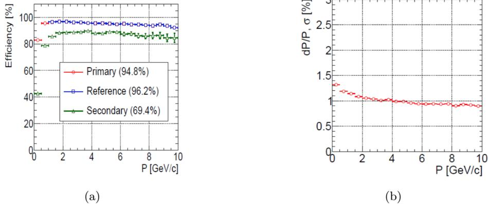
Figure 5: Track reconstruction efficiency (a) and momentum resolution (b) in the STS as a function of momentum for all tracks in central Au-Au collision at 25 AGeV.
