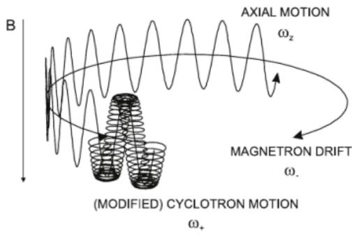
$$\begin{aligned}\omega_c^2 &= \omega_+^2 + \omega_-^2 + \omega_z^2 \\ \omega_c &= \frac{qe}{m_{\text{ion}}} B \\ \omega_L &= \frac{g e}{2 m_e} B \\ \frac{\omega_L}{\omega_c} &= \frac{g}{2q} \frac{m_{\text{ion}}}{m_e}\end{aligned}$$
