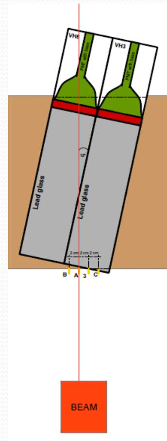
beam rotated by 12° with respect to module axis – position A
