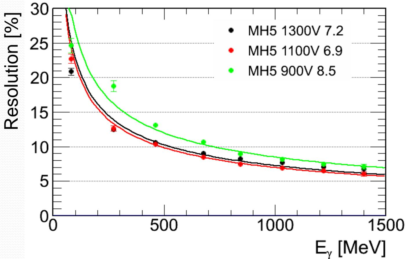
Nominal HV for 1 inch Hamamatsu to get the same pulse high as from 1.5 and 3 inch PMTs is -1300V.
