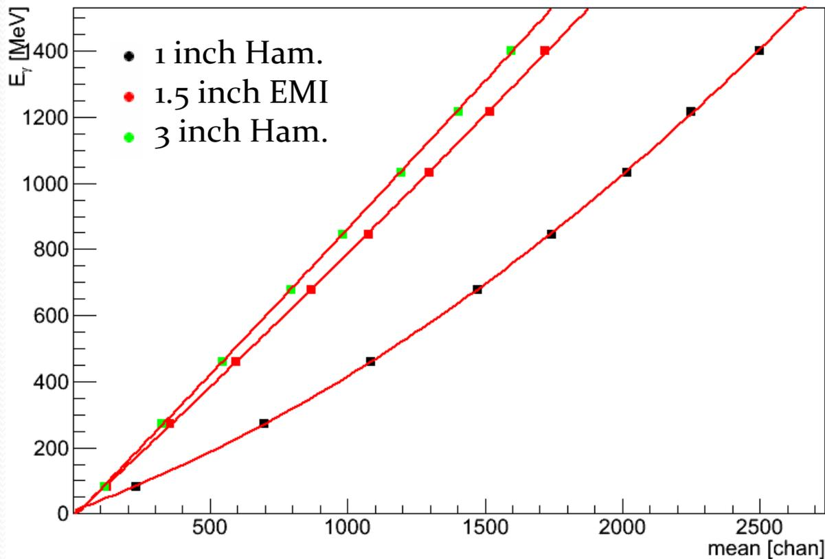
all detectors at nominal voltage (1" Hamamatsu close to maximal – saturation effects)
