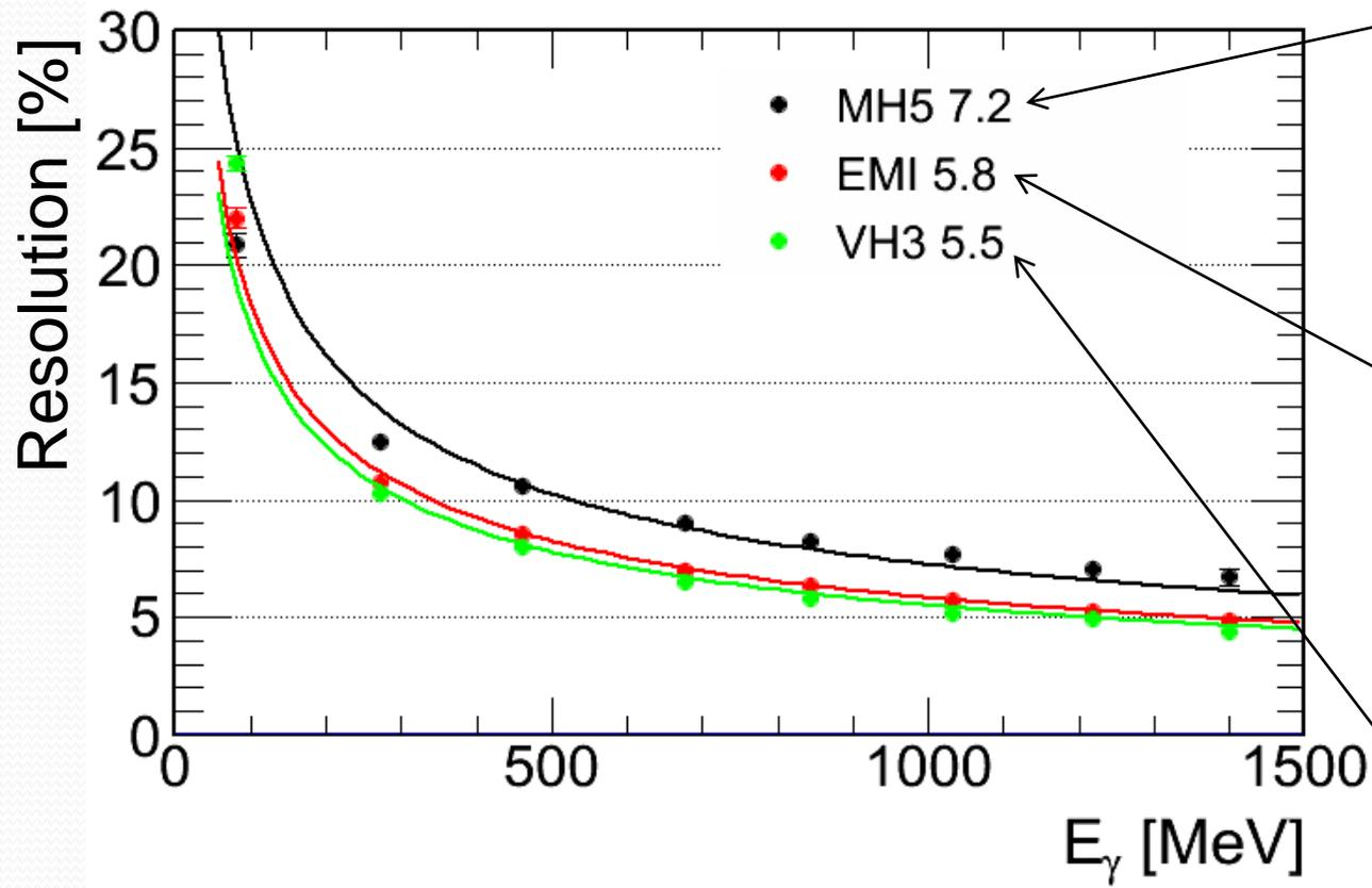
measured with CAEN ADC, signal shaped by MA8000 shaper
