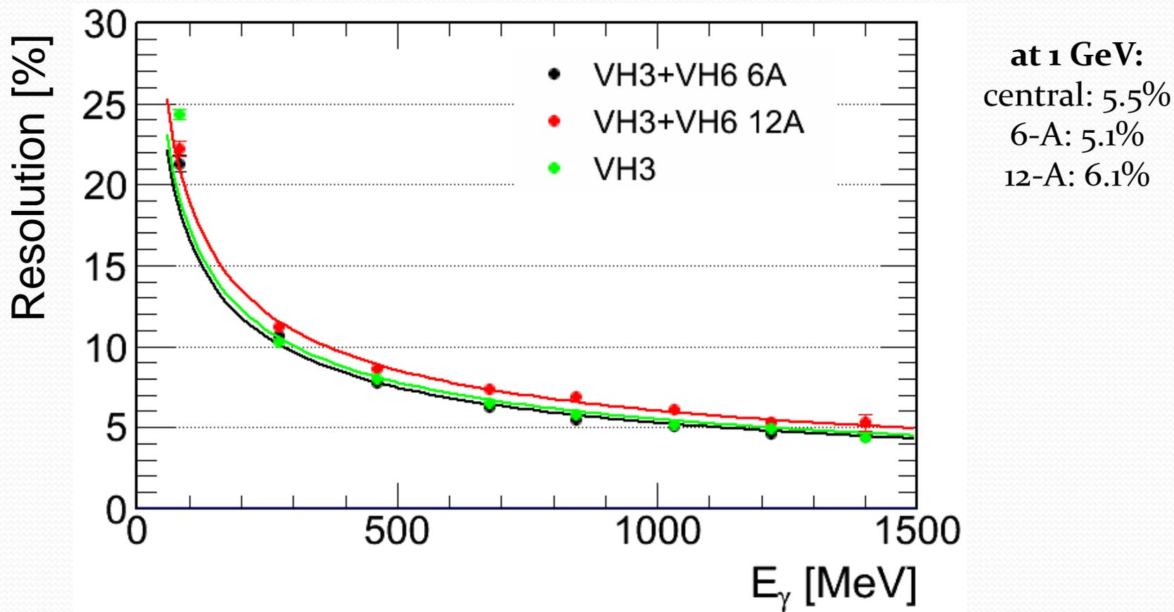
Path length in VH<sub>3</sub> for 6-A is 26 cm, path length in VH<sub>3</sub> for 12-A is 13 cm.
