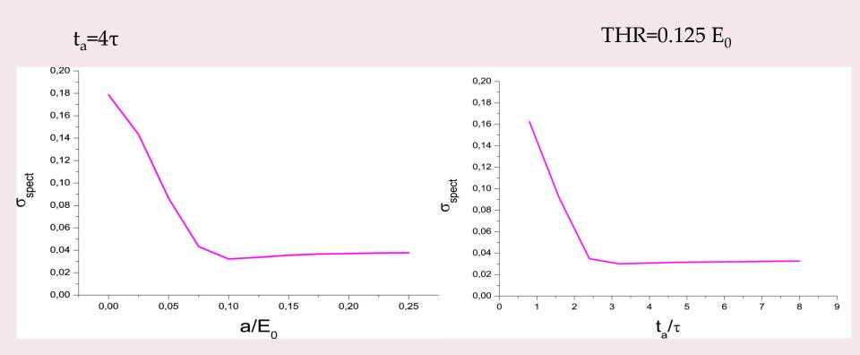
Instead of simultaneosly adapting a and  $t_{a,}$  choose the values of a and  $t_{a}$  for the highest energy in the spectrum!
