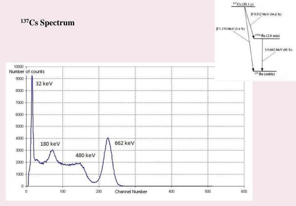
Step 1. Deduce a reference spectrum (At lower pulse frequency)
