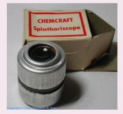
The detection of ionizing radiation by the scintillation light (produced in certain materials) is one of the oldest techniques used .
