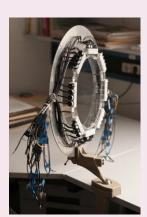
Plastic scintillator Time-Of-Flight system. (PANDA)
