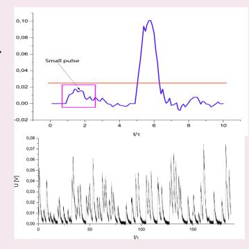
Solution – Raise the trigger by a finite value and for a finite amount of time after each pulse.
