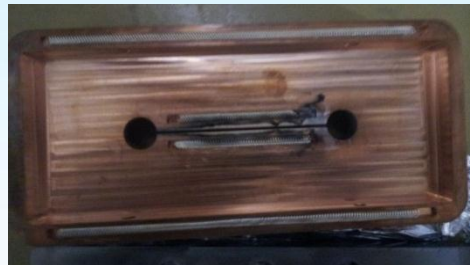
Back of Iris plate after arcing
