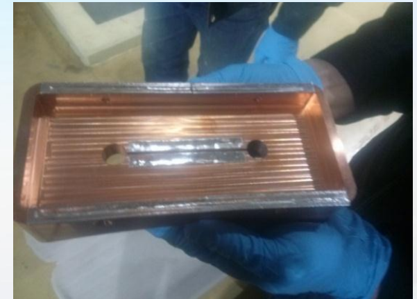
Canted coil RF seal with indium sheet (0.3 mm) to fill the gap
