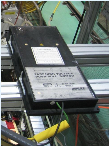
HV switch : 65kV, BEHLKE, German
