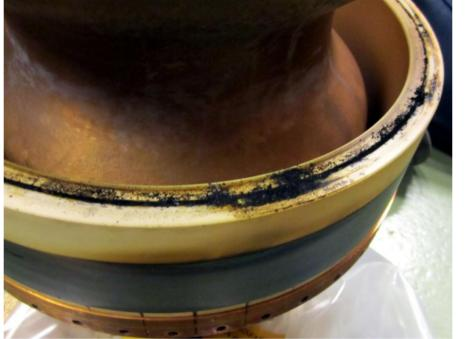
Remains of the O-ring on the cracked ceramics
