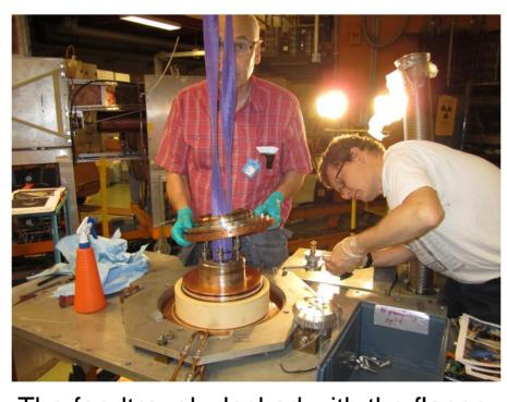
The feedtrough docked with the flange
