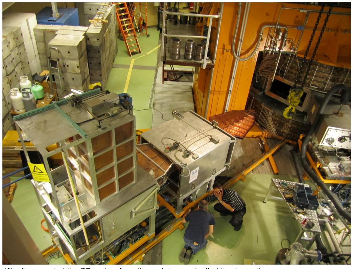
We disconnected the RF system from the cyclotron and rolled it out on rails
