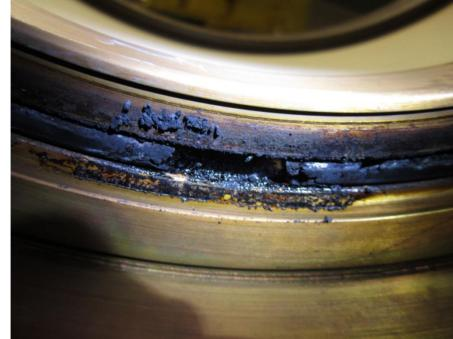
We found the main cause of the leak, a broken O-ring
