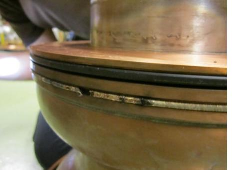
The colonial spring made of CuBe was damaged
