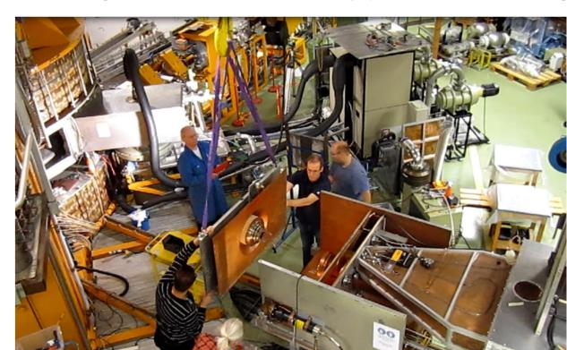
Finally the the flange with the feedthrough was loose
