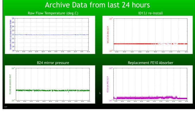
Plots cycle between the last 24 hours and the last 7 days. Archive data plots are editable so that any pv that is of current interest can be displayed. These plots are also made available via the Web pages.
