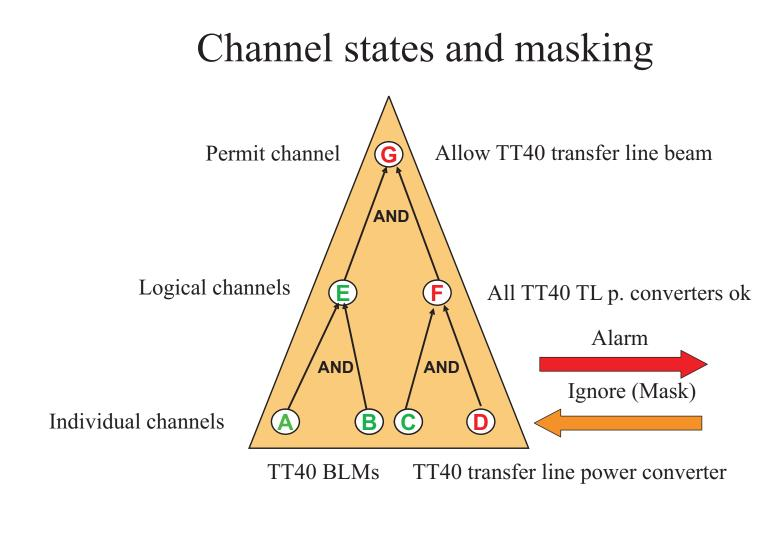
It represents a complex interlock condition on a given set of devices. Leaves are direct individual channels that are connected directly to the equipment. Intermediate nodes represents partial results (like combined power converters state). The top node is a Permit signal that gets
