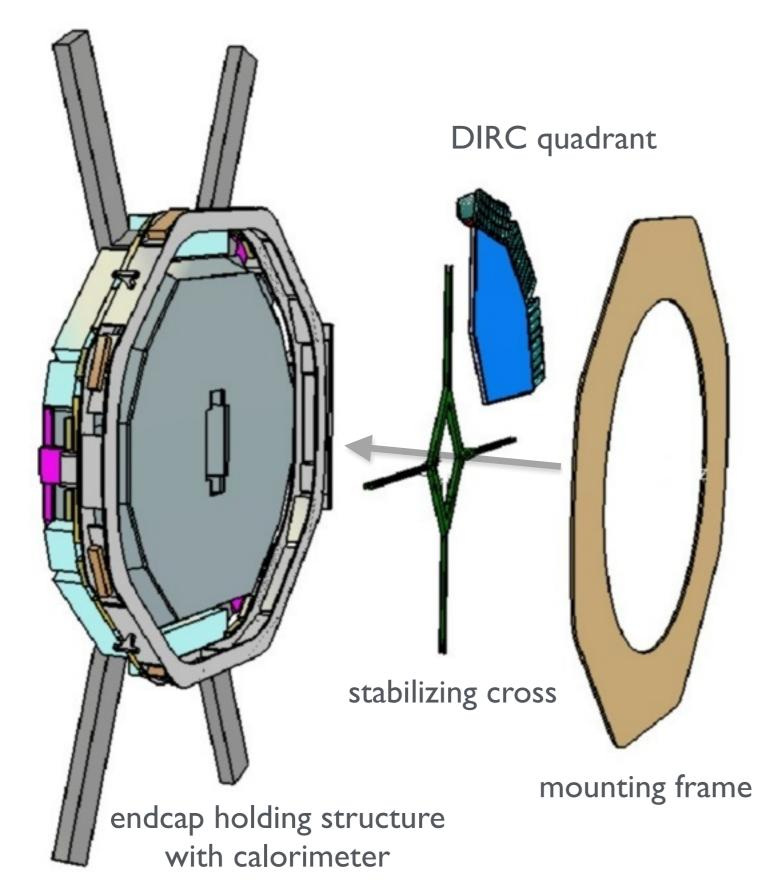
assembly of DIRC quadrants with stabilizing cross and mounting frame in horizontal position
