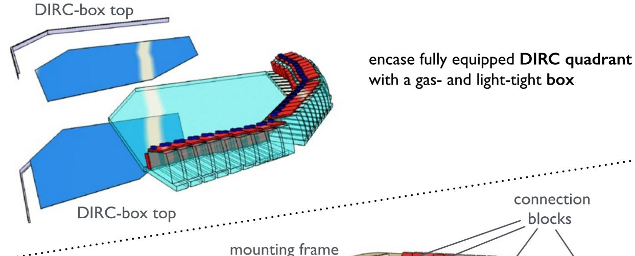
slide DIRC-box into stabilizing cross
