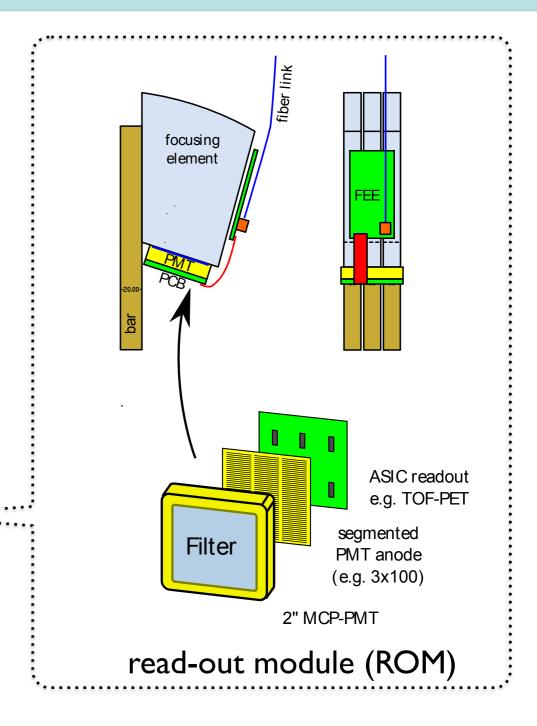
each ROM hosts three prisms and focusing light guides (FLGs) as well as a photo-sensor (MCP-PMT) and the front-end electronics (FEE)
