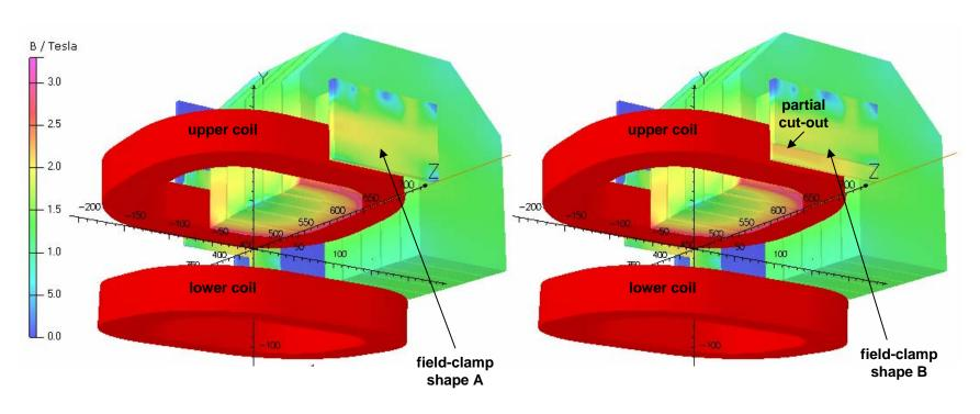
Dipole models, view from the exit side. For symmetry reasons only one quarter of the iron was considered. Where the color is yellow the field in the iron is 2 Tesla.
