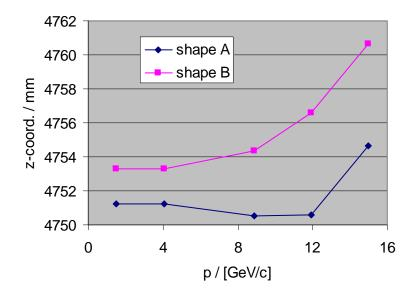
For shape A, the z-position of the VDP changes from 4751 mm @ 4 GeV/c to 4755 mm @ 15 GeV/c. For shape B, the z-position changes from 4753 mm @ 4 GeV/c to 4761 mm @ 15 GeV/c.
