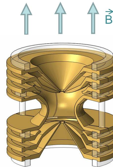
The free cyclotron frequency is inverse proportional to the mass of the ions!
