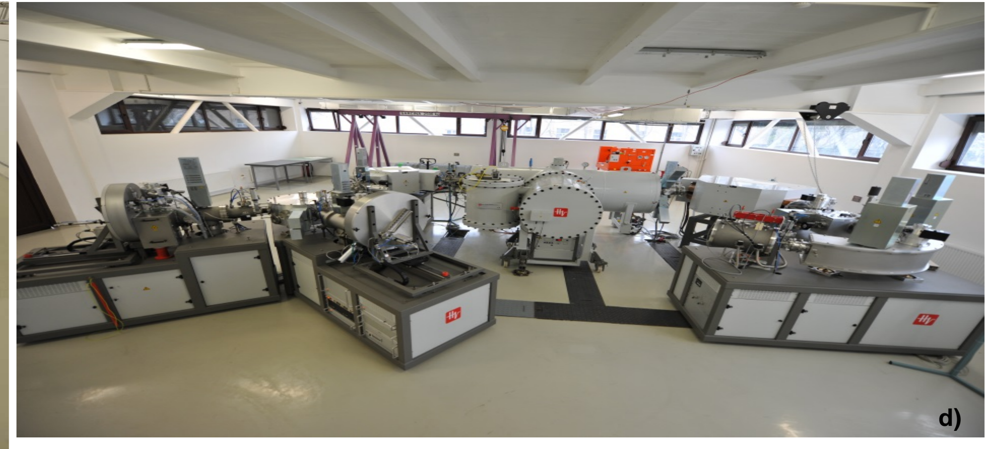
c) the 3MV Cockcroft-Walton Tandetron accelerator for IBA d) the 1MV Cockcroft-Walton Tandetron accelerator for AMS and C-14 dating
