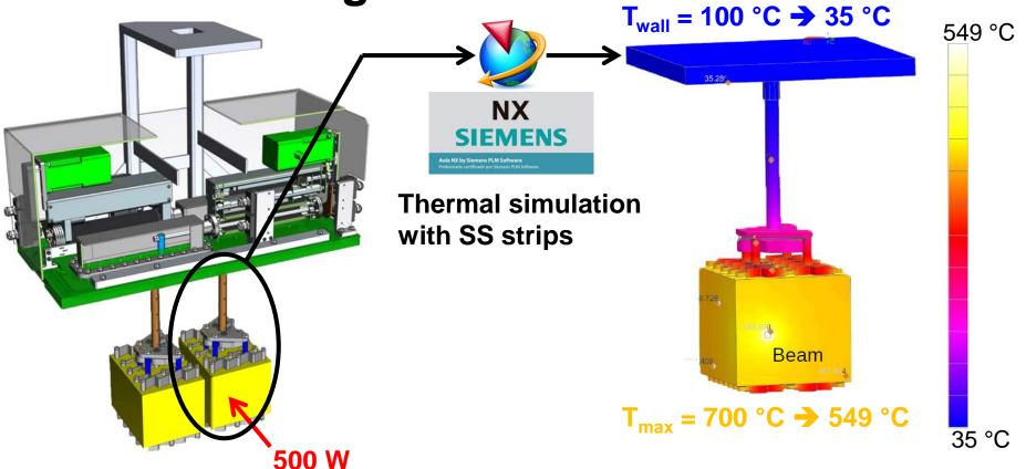
NX simulation: electronics are safe at 35 °C Will the electronics be safe in the real world too?
