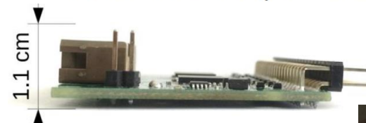
New FEBv4 (with temperature sensor & chip e-ID)
