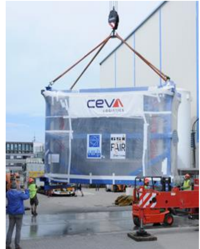
Whole OT in transport frame, 7x5.5x3.5 m 3 , 24t, arrival at GSI, Aug. 25, '23. (Photo courtesy: GSI)
