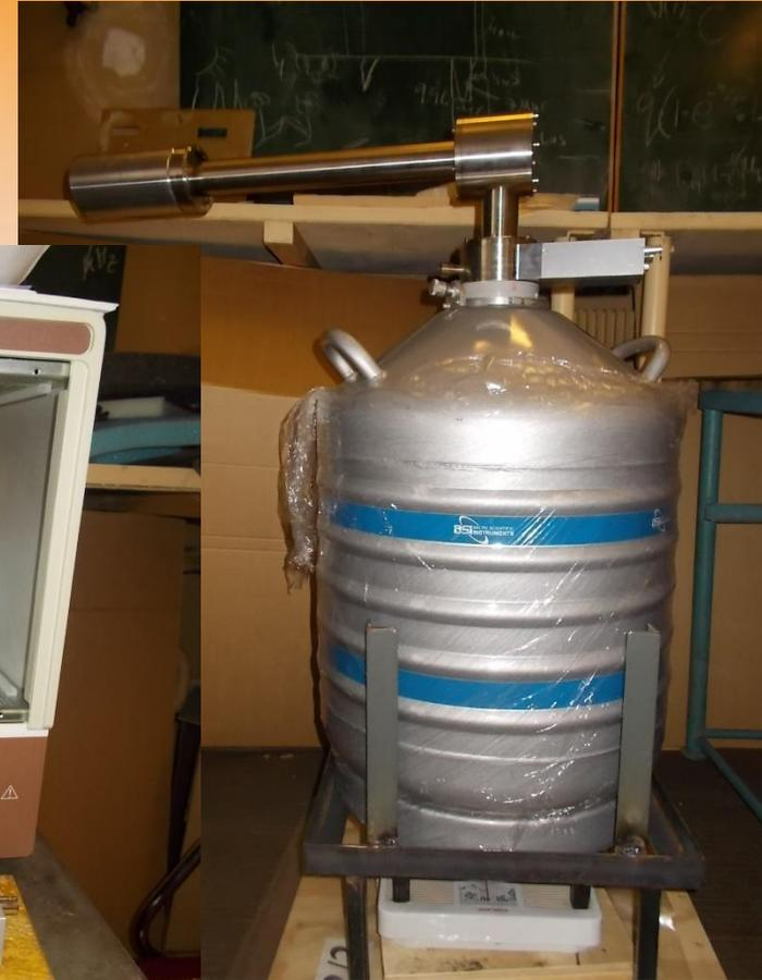
The energy resolution of DBGL spectrometer at LEPTA project is 1.2 keV interpolated at 511 keV.
