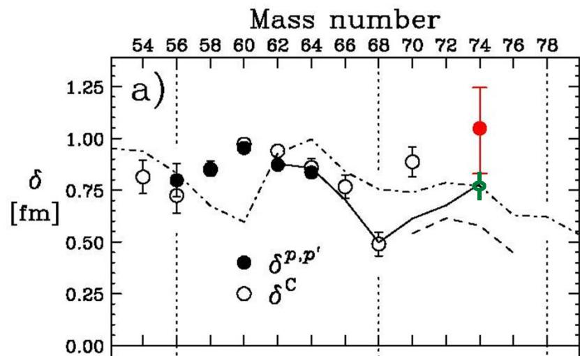
Inelastic scattering data compared to Coulex results allow to disentangle the proton/neutron excitation matrix elements. For the <sup>74</sup>Ni isotope, their difference could be an indication of the relative proton/neutron cores polarization leading to different deformation. A higher degree of accuracy is needed to constrain the B(E2) error bar and provide quantitative Mn/Mp ratio information.
