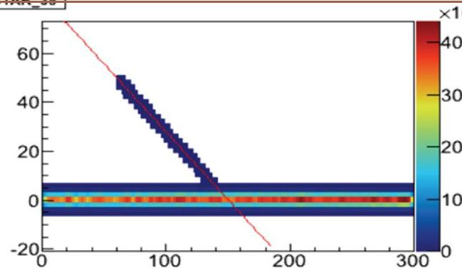
**Fig. 4:** Sample digitized trace for a  $^{132}\text{Sn}(\text{d},\text{p})$  reaction with  $2 \times 2 \text{ mm}^2$  sized pads. The red line corresponds to the fitted trajectory used for determining the range of the proton.
