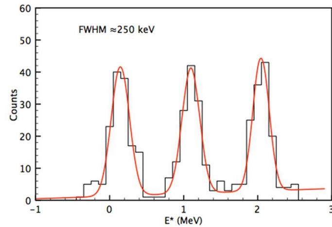
Proton energy resolution for the  $^{78}\text{Ni}(\text{d},\text{p})$  reaction at 8 AMeV with  $4 \times 4 \text{ mm}^2$  pads
