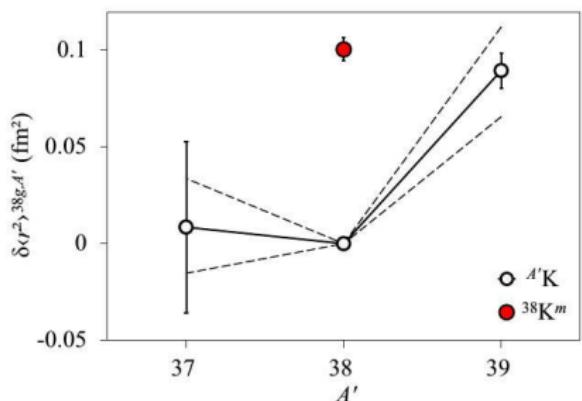
FIG. 2. Changes in mean square charge radius referenced to  $^{38}\text{K}$ . The systematic uncertainty related to the atomic specific mass shift is represented by the two dotted lines. Datum for  ${}^{37}\text{K}$  taken from [23].
