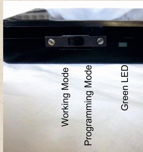
Mode switch and LED (LED off – Working Mode, LED on – Programming Mode)
