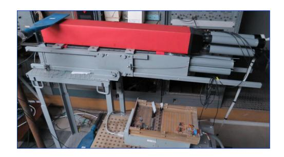
All prototype modules will be tested with cosmic muons before shipment to Giessen
