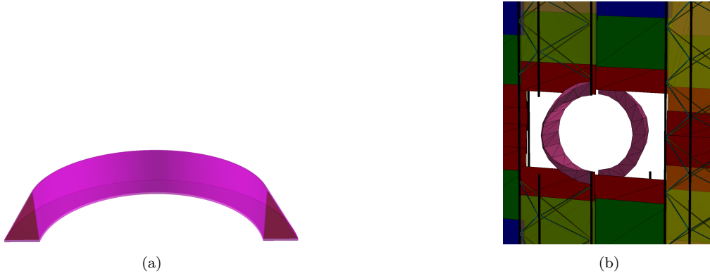
Figure 2.7: CBM-STS views: Figure 2.7a Hollow curved rib for the central ladders prepared using TGeoPcon 2 primitive solid using ROOT and Figure 2.7b Central ladder along with curved rib in STS simulation geometry.
