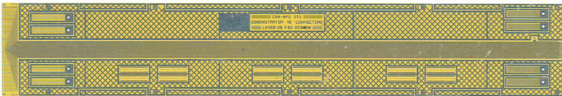
Figure 2.8: Top view of the micro-cable of length 60 cm.
