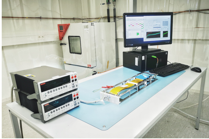
Figure 4.3: Test station for the IV measurements. The two Keithley 2400 power supplies and the computer station with the LabVIEW application for controlling and monitoring are shown.
