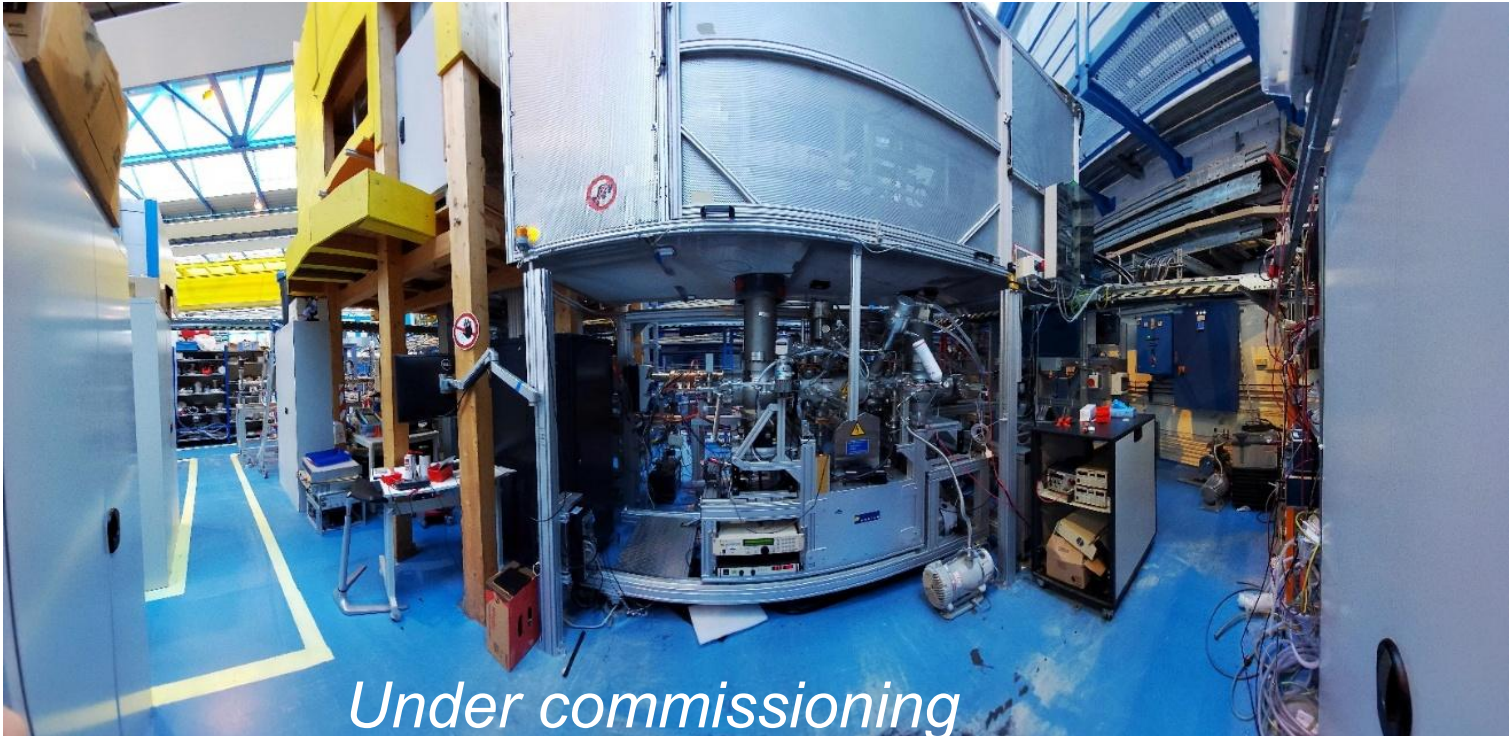
Ion source S-EBIT II for local operation of HITRAP experiments. Ions up to U^{89+} can be produced. Provided by Stockholm Univ. and HI Jena. Currently, limited to 10 kV operation voltage.
