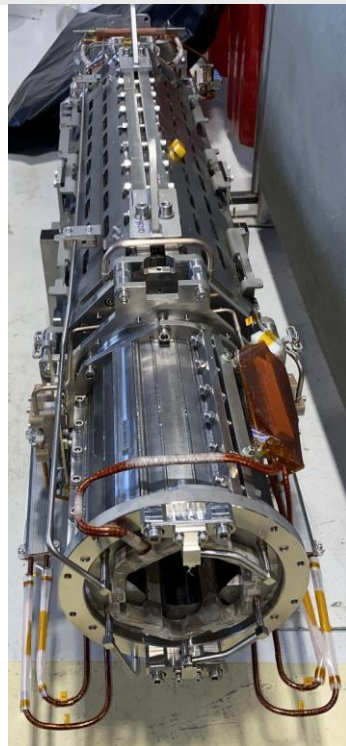
BNET36 industry prototype quadrupole unit
